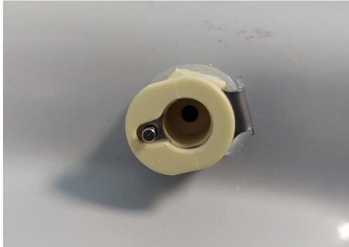
Figure 1: Leak test socket in the bowl
